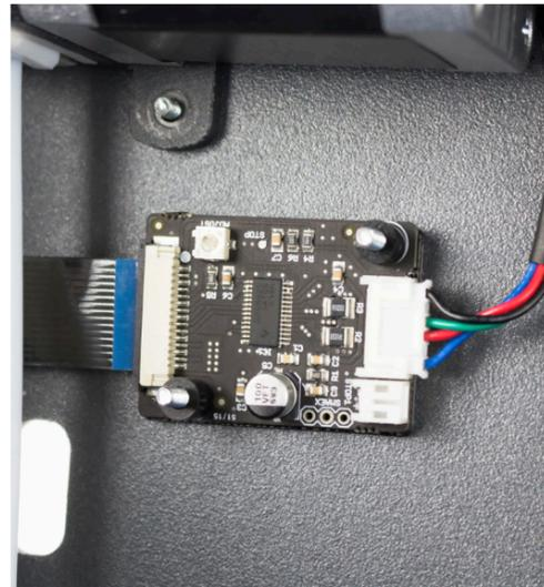
19. Connect the flat cable to the new Driver. Then place the Driver with the same back spacer and connect the Stepper motor wire.
